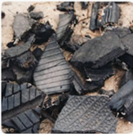
Rubber Rock (shredded tire chips) is used in place of gravel in septic system drain fields.
